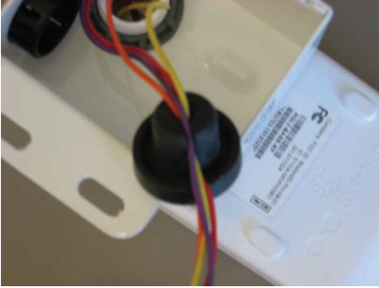
STEP 13: Add rubber plug to base station cable.
