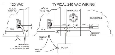
Note: Wire the pump directly to the timeclock--do not use the Aqua Rite Pro as a junction box.
