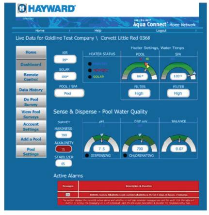
All of the information on the Dashboard is also available on the Remote Control page, but you have to either look for it in the menu structure or wait for it to appear on the two line text display. The Dashboard is a convenient display of a lot of information simultaneously.
