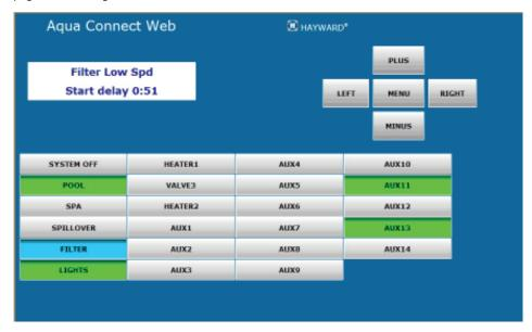
Note that there is a two line text display (white background), menu navigation buttons (to the right of the text display) and pool control buttons (below the text display). The "Check System" LED is implemented as text just below the two line text display (when a Check System situation exists).
