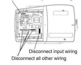
5) Remove the five screws holding the PCB in place.
