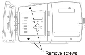
2) Swing panel open and disconnect the four conductor cable from the main PCB.
