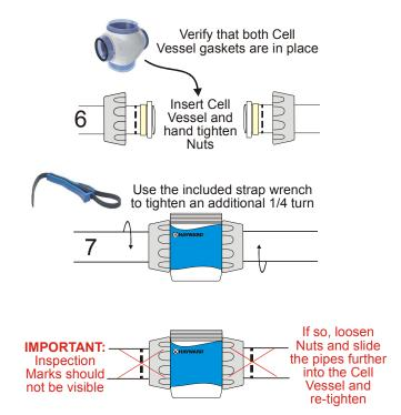
Remove the foam protector from the Cell. Verify that the O-Ring is attached before inserting the Cell into the Cell Vessel.
