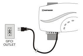
After being powered on for the first time, the Salt & Swim will run a diagnostic routine which can take up to 30 seconds. During this time, various LEDs will turn on and off. When finished, the Salt & Swim will display a blinking INADEQUATE WATER FLOW LED and a solid STANDING BY LED. Keep the Salt & Swim powered for the remainder of this procedure and go to Step 3.
