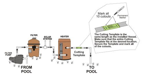
Remove the Template, cut the pipe and install the Nut Assemblies as shown below. Use the included 2" Nut Assembly for 2" pipe and  $1\frac{1}{2}$ " Nut Assembly for  $1\frac{1}{2}$ " pipe. Place Nut Assembly on each side of the cut pipe (threads face in). Be sure to place the Nut, Compression Ring and Collar on the pipe as shown in the diagram.
