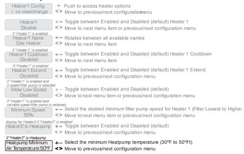
When "Heater 2" is set to Heatpump, a minimum temperature can be set. This is the minimum air temperature at which the heatpump will be allowed to be on. The default temperature is 50°F.
