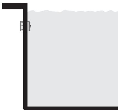
2. Drain water from pool piping. Remove flex pipe and fitting from the return jet.
