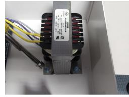
Step 5. Remove the old transformer from the can.
