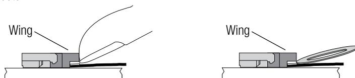
Carefully use fingernail or included plastic washer tool to lift the connector latch by the wings.
