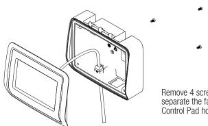
Remove 4 screws and separate the face from the Control Pad housing.
