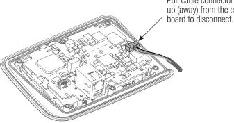
Pull cable connector straight up (away) from the circuit
