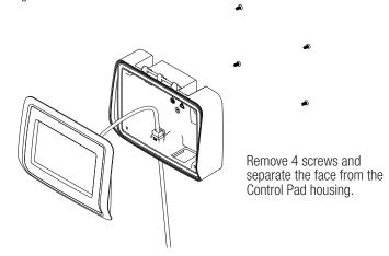
3. Disconnect RS485 cable from the printed circuit board (PCB) and discard the old housing.
