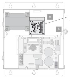
Push HLAQRPCB mounting feet firmly into holes until the circuit board is secure.
