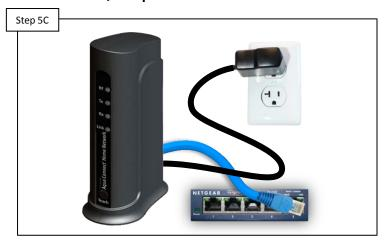
Plug the Ethernet into another router port. IF the Tx and Rx do not appear replace the Ethernet cable and if LEDs still do not appear go to Step 5D. IF LEDs appear, teach the AquaConnect (p. 8).
