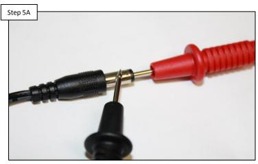
Unplug the power cable from the back of the AquaConnect and test for 5V<u>DC</u>. IF 5VDC is NOT present, proceed to step 5B. IF 5VDC is present, go to step 5C.
