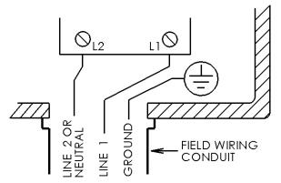
**ATTENTION:** ROUTE WIRING DIRECTLY FROM FIELD CONDUIT TO TERMINAL BLOCK AS SHOWN. DO NOT BUNDLE EXCESS WIRING INSIDE DRIVE ENCLOSURE.
