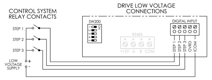
Connection wire must be rated for a minimum of 300V. Inputs are rated to accept a low voltage supply of 18-30VAC (24VAC+/-20%) or 9-30VDC (12/24VDC +/-20%). The "+12V" and "COM" terminals may be used as a low voltage supply, however, these terminals also supply power to the user interface, so care must be taken when connecting to these terminals to ensure proper operation of the user interface. SW200 DIP switch #1 must be "ON".
