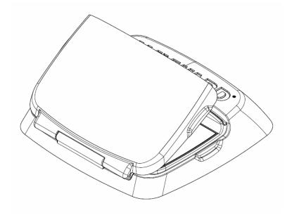
3. Align one hinge between replacement cover and bezel.
